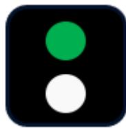
Fishing vessel with gear extending
