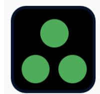
Vessel engaged in mine clearing
